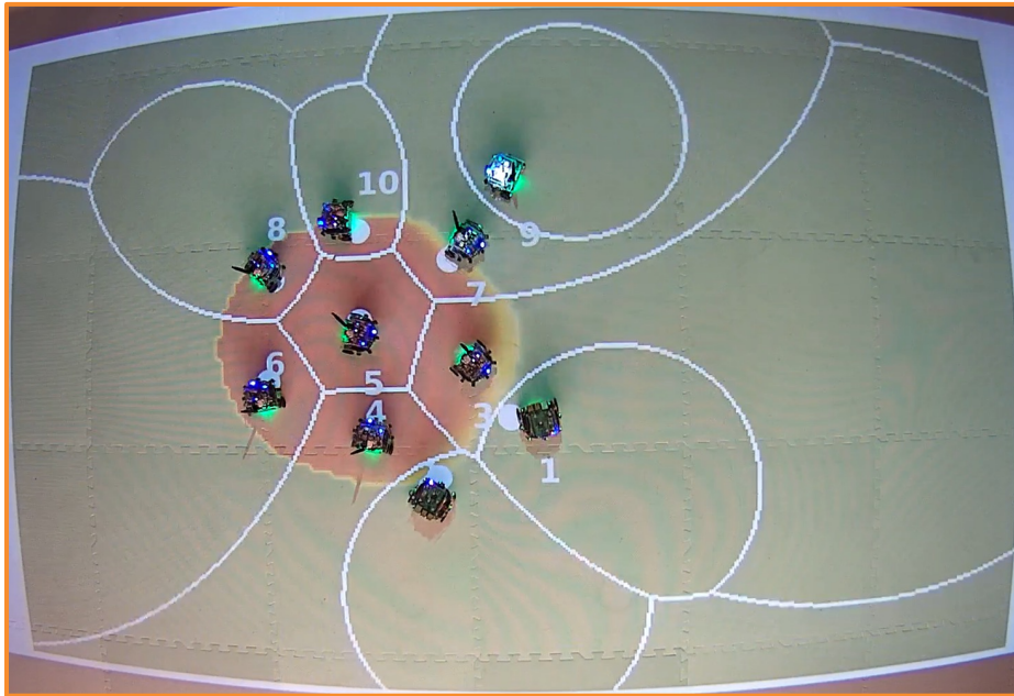
Dynamic Area Coverage with Fire-Fighting Robots [1]
